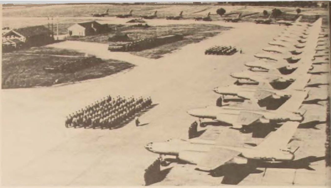
The Harbin B-5, seen here at an unnamed base, is the backbone of the Chinese bomber force. Derived from the Soviet 11-28, which first flew in 1948, the B-5 is still being produced in China. The PLAAF probably has about 400 B-5s in service. Maximum bomb load is about 6000 pounds.
